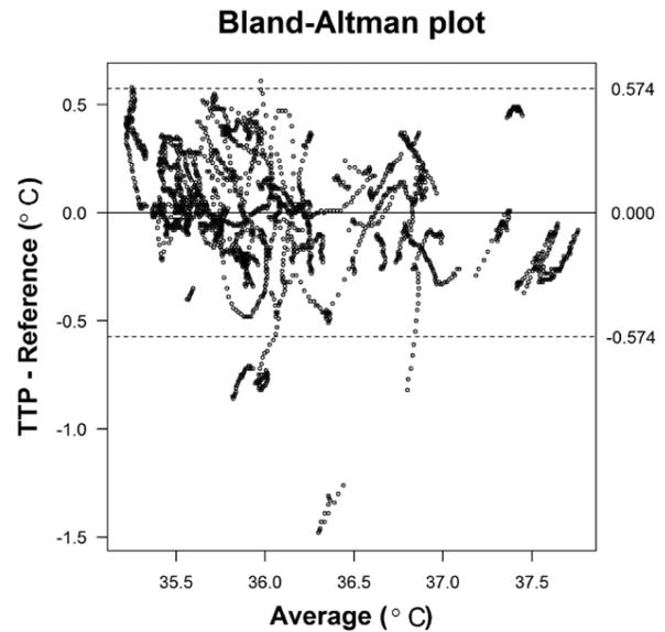
**Figure 3.** Bland-Altman plot of core-temperature measurements using the Temple Touch Pro (TTP) system versus an invasive probe. Limits of agreement (dashed lines) on the plot indicate where 95% of differences between the 2 methods are expected to fall.
