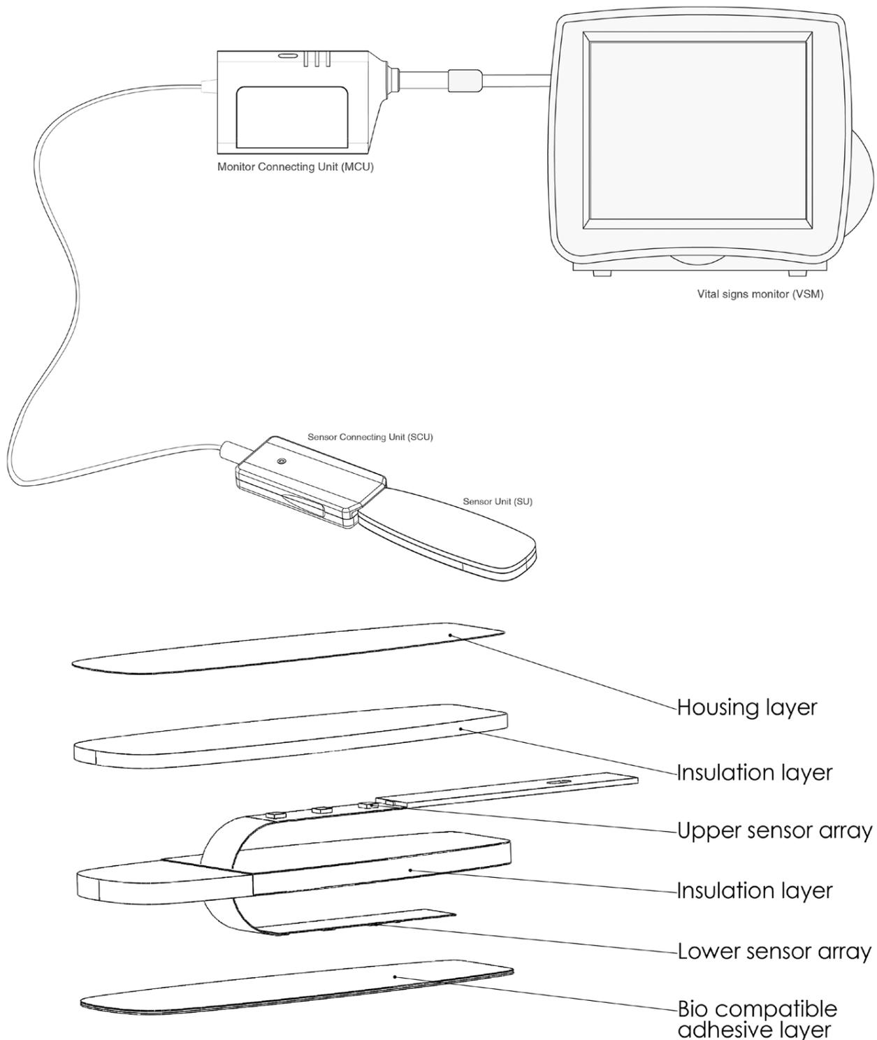
**Figure 1.** Illustration of the Temple Touch Pro system, with close view on the sensor layers.
